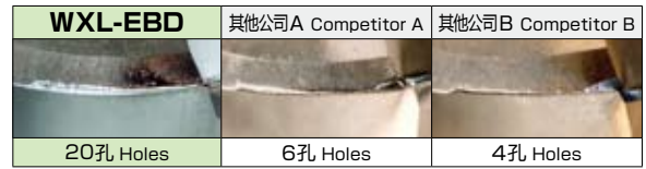
加工后的磨损状况 Tool Wear After Milling
