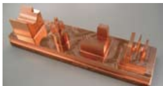
电极模具加工 Electrode model milling
