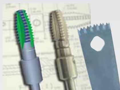
Dental taps. Following accurate 3D simulation, the parts are ground on the machine. What you see is what you get.
