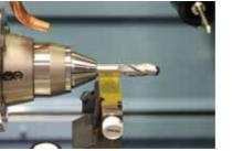
• P-axis traveling steady for use with bush or hydraulic Arobotec
